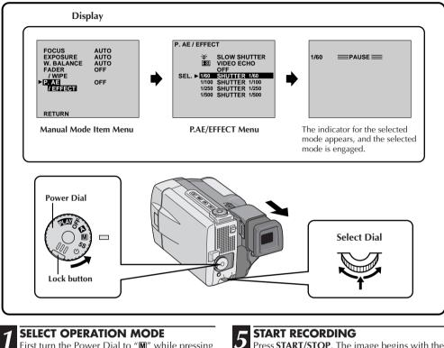
First turn the Power Dial to "M" while pressing down the lock button located on the dial. make sure the LCD monitor is open fully or the viewfinder is pulled out.
